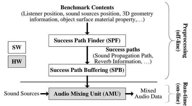
Figure 1. Overall architecture of proposed audio mixing system
