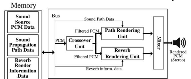
Figure 2. The proposed AMU H/W architecture
